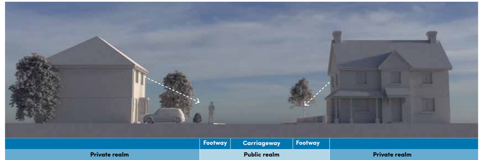
FIGURE 36. Typical section through the Residential Street
