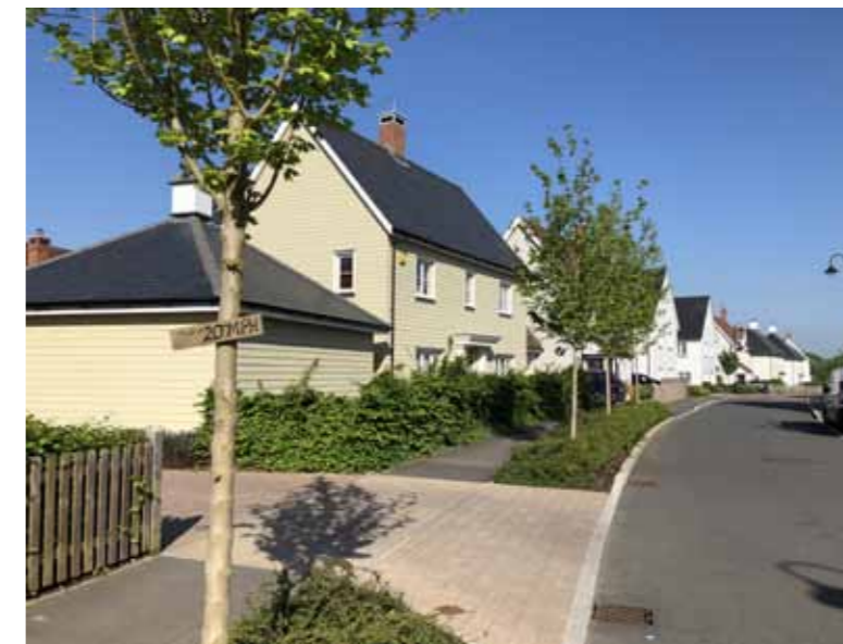
Street trees and planting within verges to separate the footway from the road
